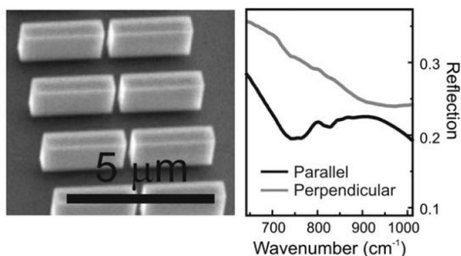
Fig. 1. A SEM image of the Ge antennas on Si (left panel) and sensing of the  $800 \text{ cm}^{-1}$  vibrational line in PDMS (right panel) for polarization parallel (black line) and perpendicular (grey line) to the antenna axis).
